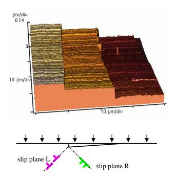
**Figure 1** – An Atomic Force Microscope image of a cleaved LiF single crystal. The surface ledges, under contact, will emit dislocations along certain slip systems, as shown schematically.
