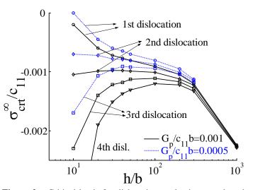
**Figure 2** – Critical loads for dislocation nucleation are plotted against the step height h/b (normalized by b, the magnitude of Burgers vector). This plot only considers the slip plane L.
