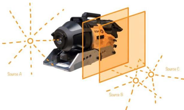
Fig. 12. Schematic of detector, sources, and shielding arrangement. [2]
